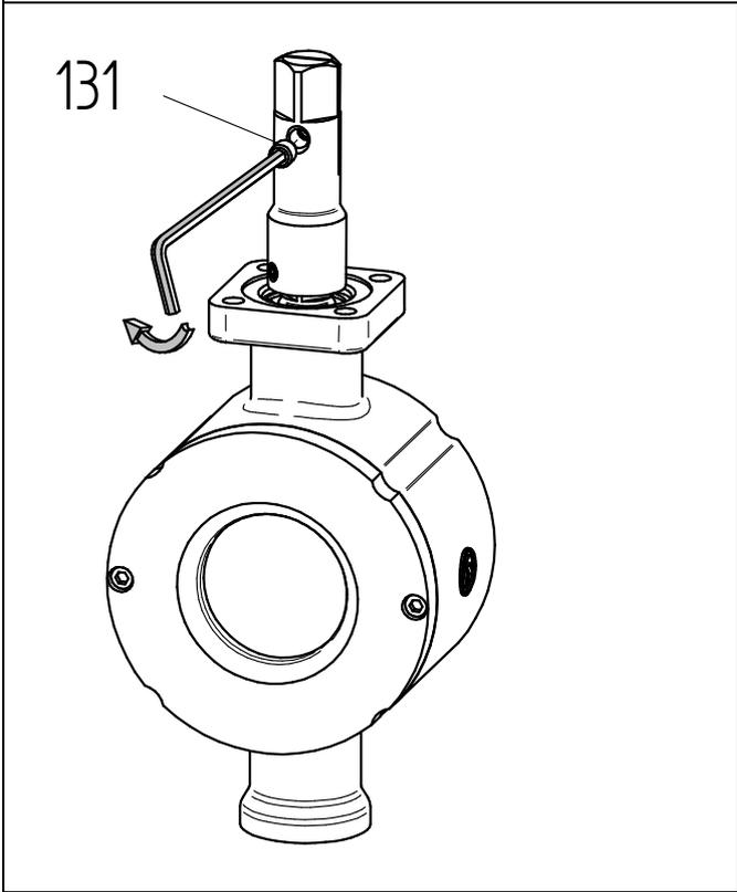
✓ Screw the screw pin (131) in loosely
