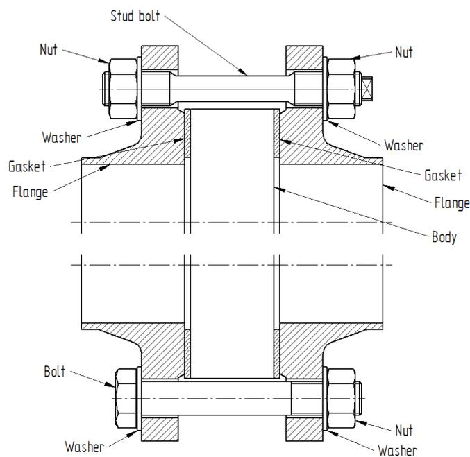
The threads of the bolts must be greased. The bolts must be tightened crosswise. Apply 30% of the nominal tightening torque with the first tightening sequence, 60% with the second and 100% with the third. The procedure should then be repeated with 100% of the nominal tightening torque until the nuts cannot be turned any further when applying the nominal tightening torque.
