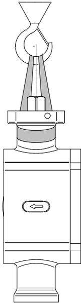
Retaining points for valves with an actuator
