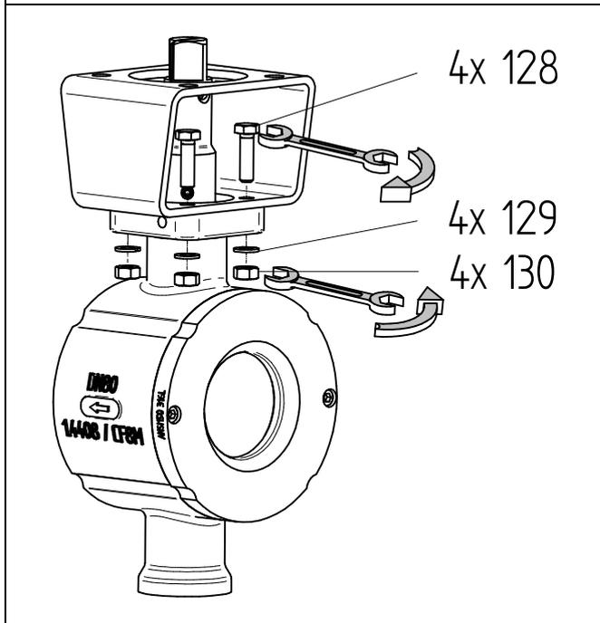
✓ Screw the console on tight using 4 hex. screws (128), 4 washers (129) and 4 nuts (130)
