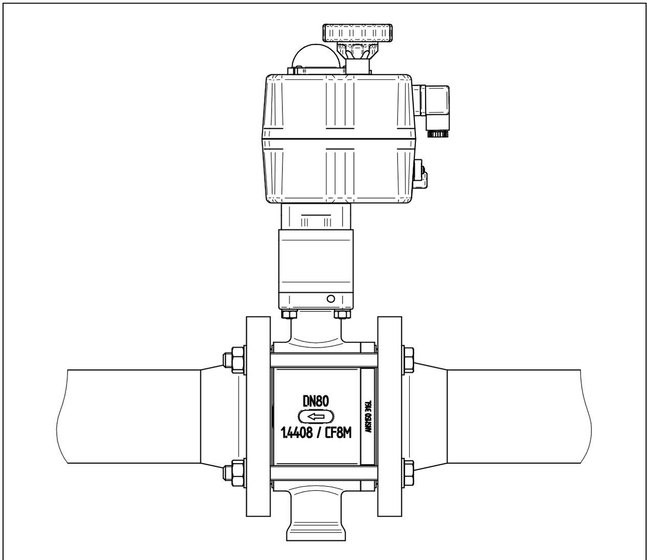
The valve is inserted between two flanges. Seals conform with EN 1514-1 or ANSI B16.21 respectively with the required pressure level are to be positioned on the sealing surfaces. Serrated metal gaskets, spiral wound gaskets or other gaskets with metal rings are not suitable. We recommend flange seals from pure graphite with a stainless steel insert.
