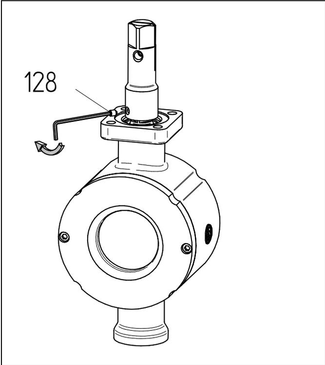
✓ Fix the square adapter in place using the screw pin (128)
