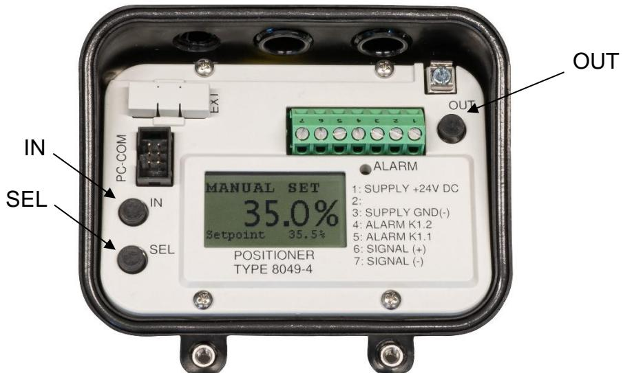
The "Manual setpoint setting" is switched off by briefly pressing the IN and OUT keys. The valve returns to the initial position according to the control signal applied.
