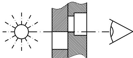
3. Lower the valve spindle further until the correct overlap is obtained.
