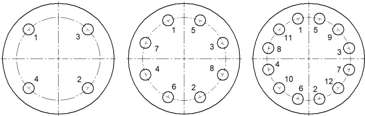
The required bolt tightening torques depend on the flange gasket that is being used. The exact values are to be taken from the corresponding data sheets or requested from the gasket manufacturer.
