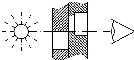
3. Lower the valve spindle further until the correct overlap is obtained.
