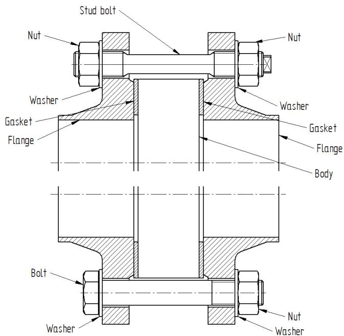
The threads of the bolts must be greased. The bolts must be tightened crosswise. Apply 30% of the nominal tightening torque with the first tightening sequence, 60% with the second and 100% with the third. The procedure should then be repeated with 100% of the nominal tightening torque until the nuts cannot be turned any further when applying the nominal tightening torque.
