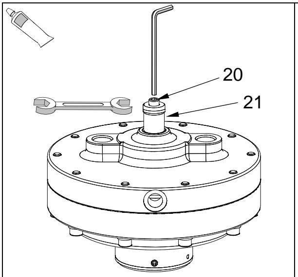
12. Lock position of regulating nut (21) with screw pin (20).
