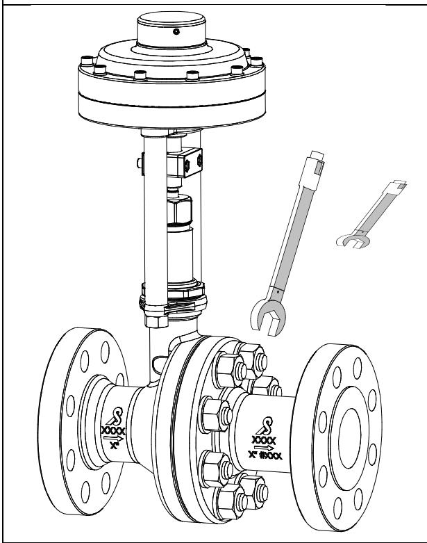
23. Set the torque wrench to the appropriate torque.
