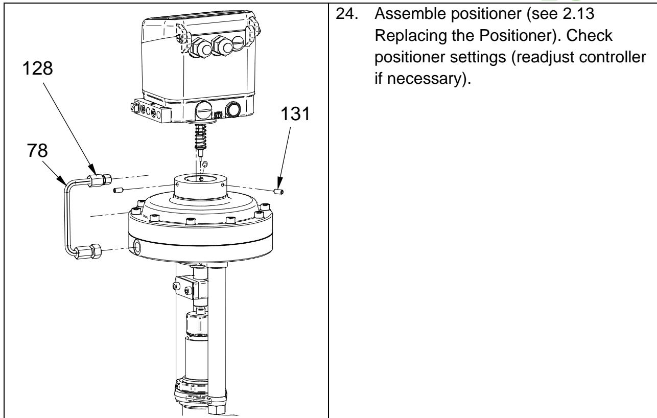
24. Assemble positioner (see 2.13 Replacing the Positioner). Check positioner settings (readjust controller if necessary).
