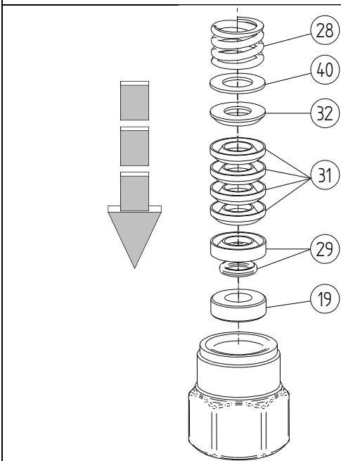
3. Insert complete packing into tube (16) using a suitable tool. Take care to assemble in the right order.
