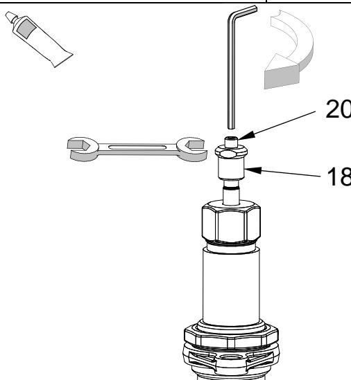
12. Lock the position of the regulating nut (18) with the screw pin (20).
