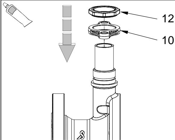
2. Insert washer for column (10) in the correct orientation and tighten nut (12).
