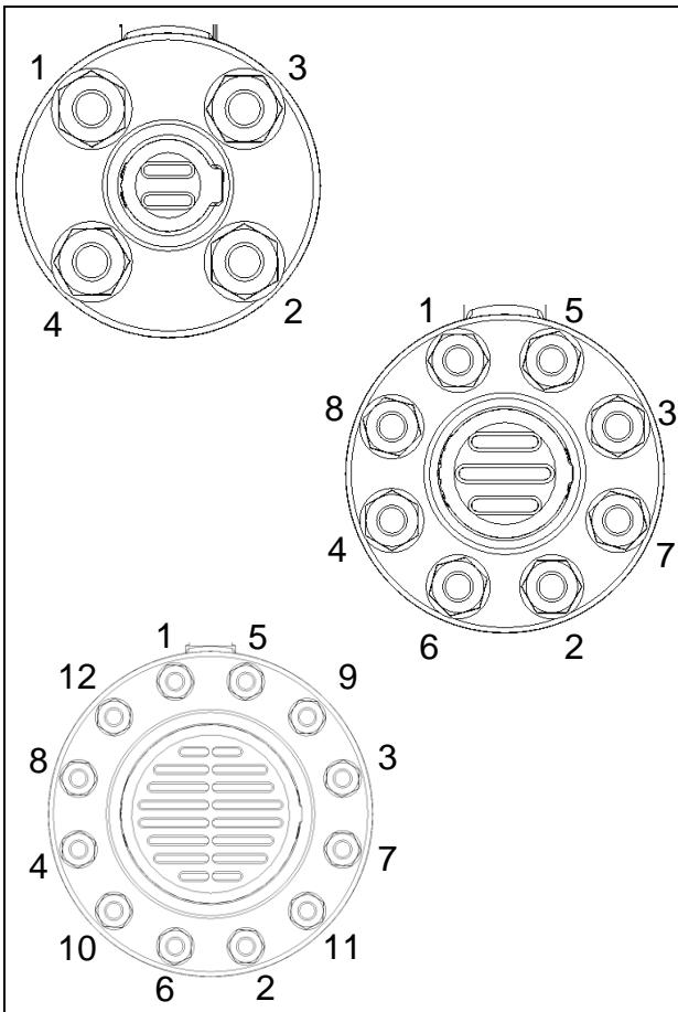
21. Tighten the nuts (221) with the cross pattern shown on the left.
