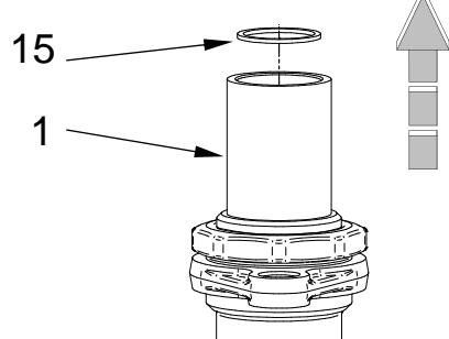
10. Remove seal (15) from valve housing (1).
