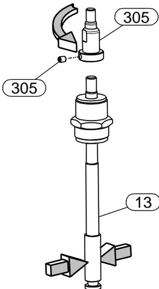
12. Carefully clamp the valve stem (13) at its lower section.
