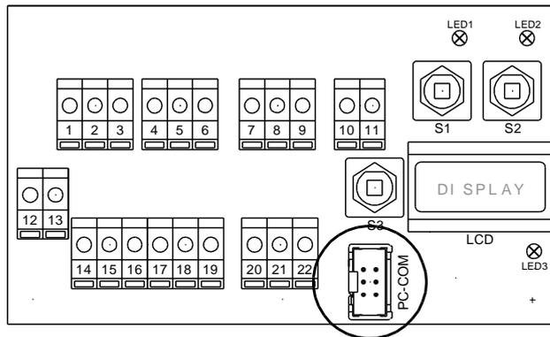
The connection to a PC is made by using a special adaptor at the “PC-COM” connection in the terminal compartment of the actuator.
