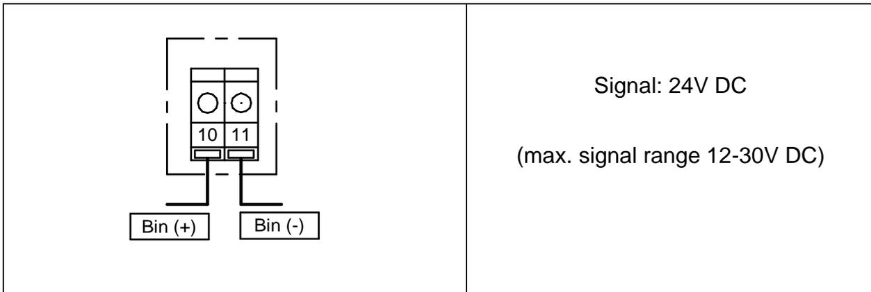
The binary input overwrites the set point signal present and executes the stored special function.
