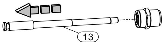
15. Pull the valve stem (13) from the packing. Press the guide sleeve (19), packing (299), washer (40) and spring (29) out of the packing tube.
