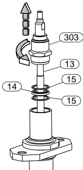
10. Unscrew packing tube (303) and pull it from the body (1) together with the valve stem (13).
