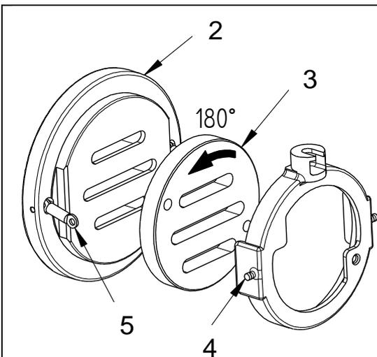
The valve's closing action can be reversed by turning the movable valve plate.
