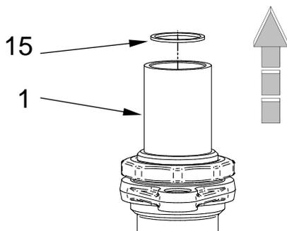
16. Remove seal (15) from valve housing (1).
