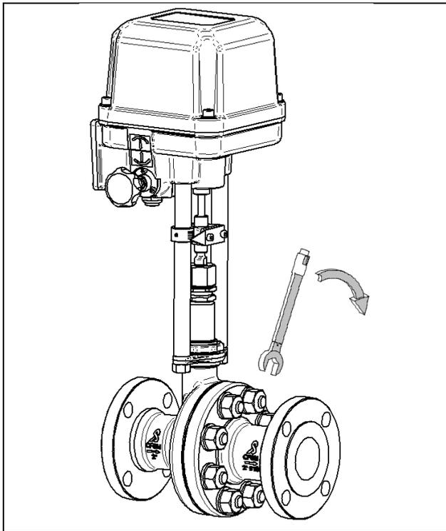
25. Set the torque wrench to the appropriate torque.
