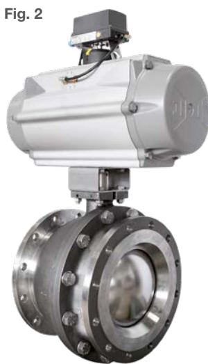
Fig. 2 Ball sector valves from the 4040 range are available in the nominal sizes of DN 25 to DN 300. Up to a nominal size of DN 250, the valves are constructed in a wafer design (in DN 300 with to PN 40 (ANSI 150 to ANSI 300). Depending on the nominal size, K_{vs} values between 1.45 and 3,840 are possible. These ball sector valves are manufactured in stainless steel 1.4408. The ball sector valves can be used at temperatures up to 220 °C depending on the selected seals.
