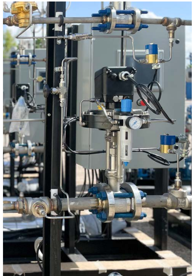
Figure 02: Due to the high rangeability of the sliding gate valve, the Thermal Well Generator now requires only one valve for gas and one for air.
