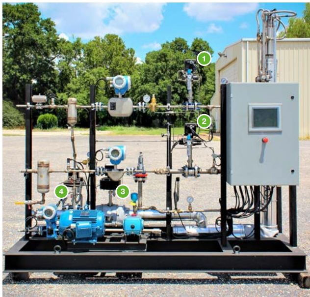
Figure 04: Multiple sliding gate valves by Schubert & Salzer are used in the Thermal Well Generator. (1) Fuel gas control valve (2) Air control valve (3) Well steam control (4) Vent steam control valve.
