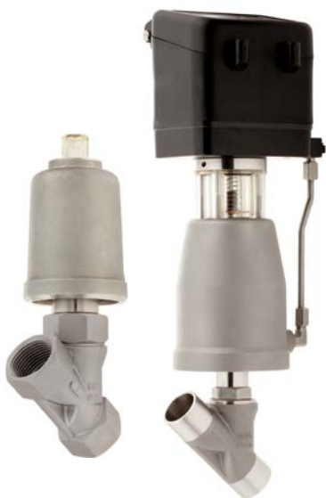
Angle seat control valves type 7020 offer high flow capacity along with bubble tight shutoff reducing the need for isolation to the process. These control valves feature integral top mount integral positioners; pneumatic, analog and digital. Angle seat on/off valves typ 7010 offer millions of maintenance free cycles in difficult applications such as steam, gaseous media and contaminated liquids.
