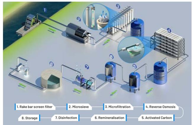
The canal water from the Ostend Canal is treated in 8 stages before being ultimately fed into the region's pipe network as clean drinking water.
